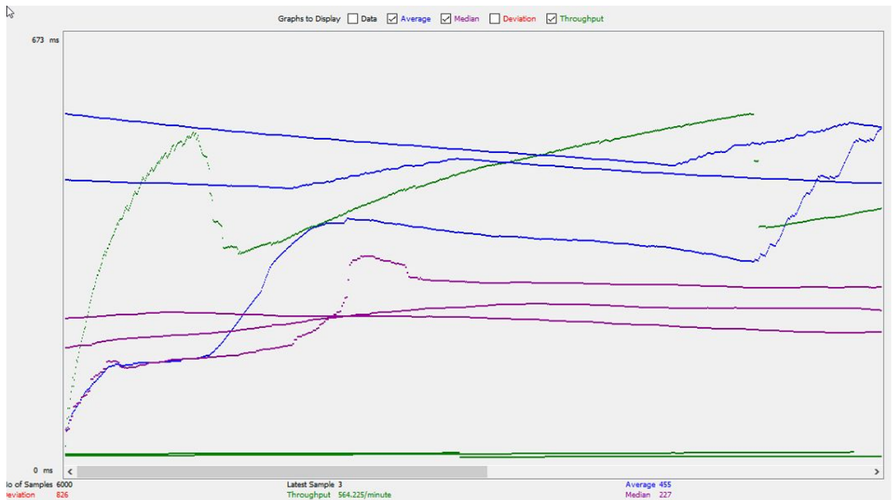
Fig 2.2 Worst results - latency average of 26 ms with a max of 738 ms
