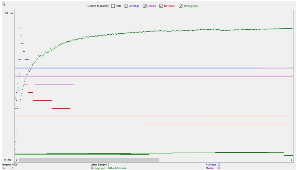
Fig 2.1 Best results - latency average remains consistently at 10ms
